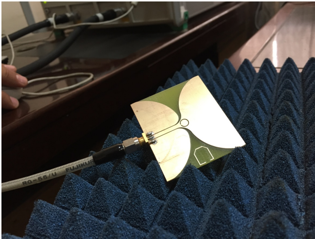
Figure 12: Measurement setup for the dual-band notch antenna.
